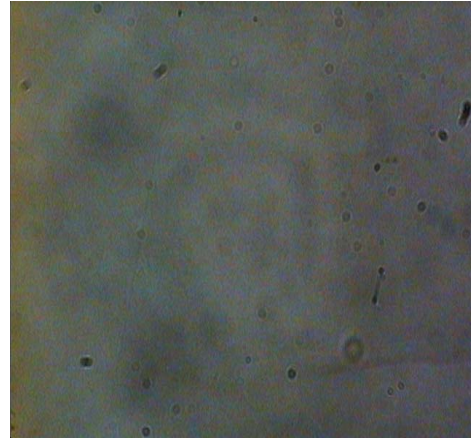
Figure 16 – Twisted-nematic cell made using corrugated glass viewed under parallel polarizers Image size: 1.13mm by 1.54mm
