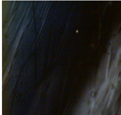
Figure 20 – Twisted-nematic cell made using corrugated glass viewed under parallel polarizers. Dark areas indicate twisted alignment and bright areas indicate parallel alignment
